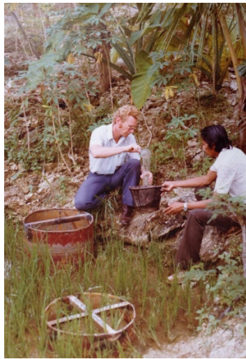
Penetration tests near Kali Bawang (testing soil conditions to assess crop water requirements for irrigation purposes)
