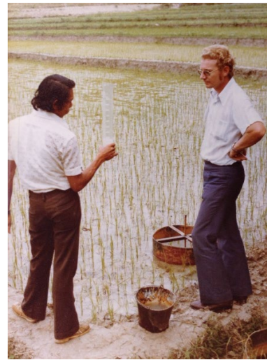
Penetration tests near Kali Bawang (testing soil conditions to assess crop water requirements for irrigation purposes)
